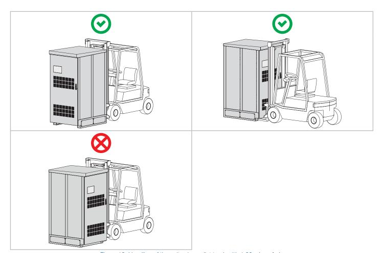
Figure 18. Handling of the unit using pallet truck with 1.30m long forks
